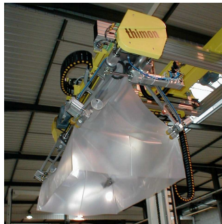
Opening and rotation of the hood for 1/2 and crosswise pallets
