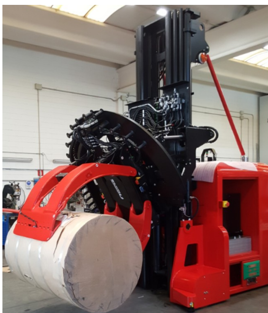
Special Clamps designed by Proxaut for tilting, rotating, shifting and lifting paper reels up to 2.500 kg (5,512 lbs)
