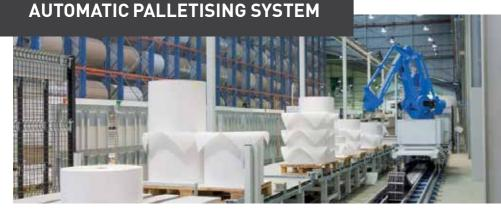
Robotic palletising systems, to palletise varying dimensions of reel, eventually feeding to an automatic wrapping / labelling system if required.
